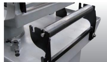
Loading side bar supporting height adjustable roller.
