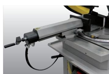
Frontal vice placed in ergonomic position made of: a thick plate supporting the clamping vice unit, a wide swiveling disk for material support (dimensioned up to the most cutting capacity) with slot for blade passage and a clamping group sliding clockwise on the plate so to allow angular right and left cuttings with quick clamping devices.
