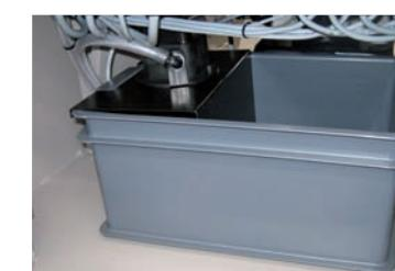
20 l coolant tank placed inside the basement easy to move for cleaning and filling.
