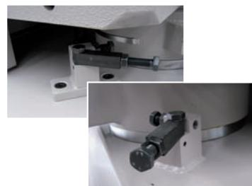
Mechanical lips for a fast head rotation at 0°, 45°, 60°, and -45°.
