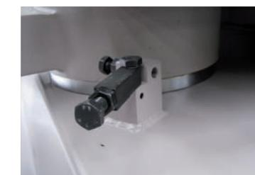
Mechanical lips for a fast head rotation at 0°, 45° and 60°.
