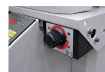
Head feeding system with hydraulic cylinder and front balanced valve for feeding regulation.
