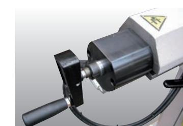
Clamping vice in cast iron movable by hand equipped with hydraulic locking cylinder.
