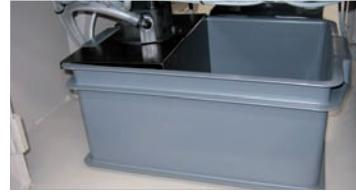
20 l coolant tank placed inside the basement easy to move for cleaning and filling.
