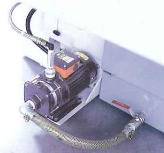
**The automatic lubrication pump is installed at low level for easy monitoring.**
